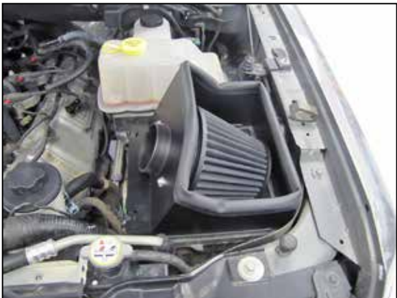
17. Set the heat shield assembly onto the lower air box and secure with the two remaining air box clips.
