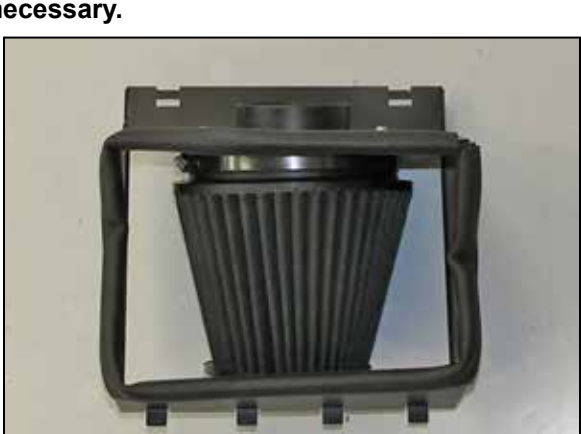
15. Install the K&N® air filter onto the adapter and secure with the provided hose clamp.
