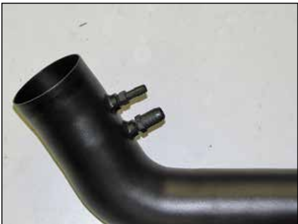
21. Install the two provided NPT vent fittings into the K&N® intake tube as shown. NOTE: NPT fitting has tapered threads and only designed to be installed until hand tight, then tighten one rotation or when the fitting becomes difficult to return.
