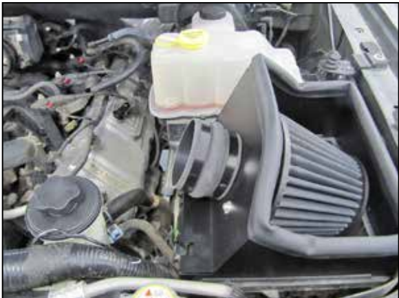
18. Install the provided hump coupler (08699) onto the filter adapter and secure with the provided hose clamp.
