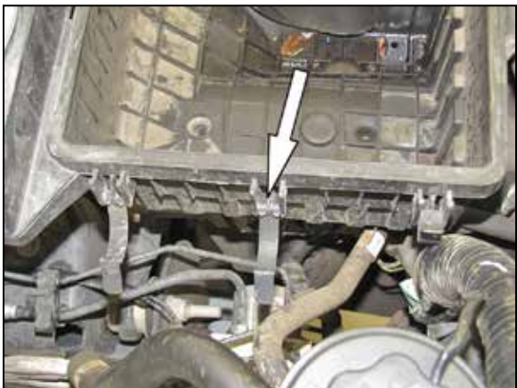
16. Remove the center upper air box retaining clip.
