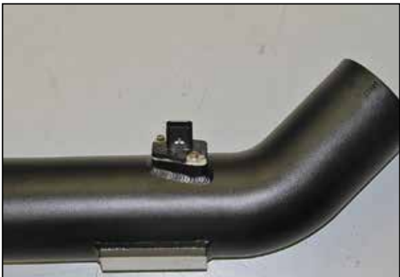
20. Install the mass air sensor into the K&N® intake tube and secure with the provided hardware.
