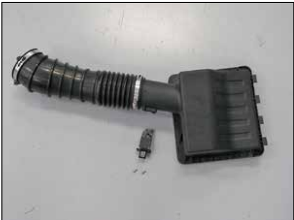
19. Remove the two screws securing the mass air sensor into the air box and then remove the sensor.
