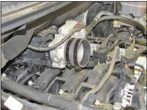
10. Install the provided coupling hose (08698) onto the throttle body and secure with the provided hose clamp.
