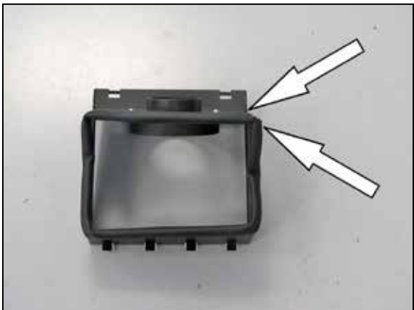
14. Install the provided "Top Bulb" edge trim onto the top of the heat shield as shown. NOTE; Some trimming of the edge trim will be necessary.
